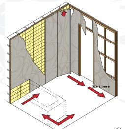
Fibo wall panels with Aqualock are fixed to battens/walls by nailing or screwing into the groove running along the length of the panel using No. 6 screws or 35mm gypsum board nails. Leave a distance of 200mm between each nail/screw. The lowest nail/screw must be fastened a maximum of 20mm from the bottom of the panel.
