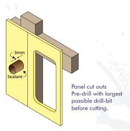
Apertures for pipes etc. The opening should have a clearance of approx. 5mm Seal the clearance with polymer sealant.
