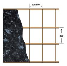
Distance between battens: Vertically - 600mm or 900mm Horizontally - 800mm
